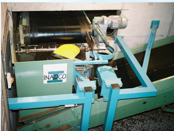
Mounting at a Corner overshoot The yellow shovel takes samples out of a vertical product stream and drops the sample in the black CEN Measuring Cylinder.
